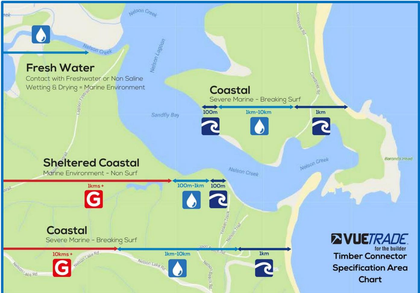
**EXAMPLE:** Say your application is near the coast: work out the type of coastal environment, the distance from the building, consult the chart and guidelines above and identify the steel grade required!
