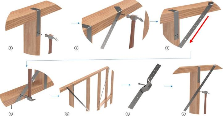
Examples are based on bracing fixing details B of VUEBRACE Builder Strapping Technical Data Sheet.
