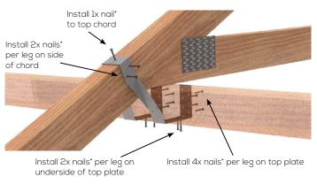
\* Use only VUETRADE 30mm x 2.8mm Ø Galvanised Connector Plate Nails for fastening Cyclone Straps.
