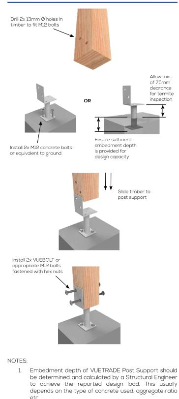
2. 75mm clearance must be provided to conform to the requirements set out by AS3660.1:2014 -*Termite management, Part 1: New building work.*
