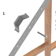
Place VUESMART Brace Tensioner on the strap and insert the screw through one of the centre holes of the strapping.
