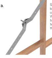
Strap bracing is a tension brace and is installed as a cross bracing. When tensioning the straps, take care to ensure even tension to avoid distorting the frame.
