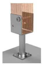
IMPORTANT: The bolts MUST be used in the designated size range, i.e. VUEBOLT 90110 must be used in working width of 90mm to 110mm. This is to ensure that there will be sufficient amount of thread between the male and female bolts to meet the minimum working strength.
