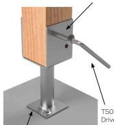
Install the FEMALE part of the VUEBOLT first and hold with one of the T50 star drive wrenches.
