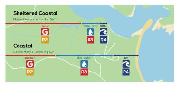
The suitability of brick ties in different environmental conditions can be determined by reading off the specification area chart based on the type of environment and the distance where the brick ties will be used.
