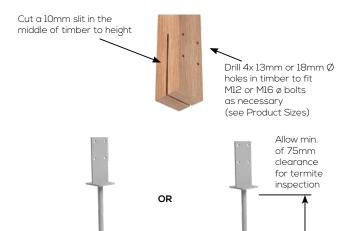
Install 4x appropriate sized concrete bolts (see Product Sizes) or equivalent to ground
