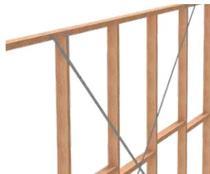
Repeat steps 2 to 4 on the other end, diagonally opposing to the first strap forming a 'X' configuration.
