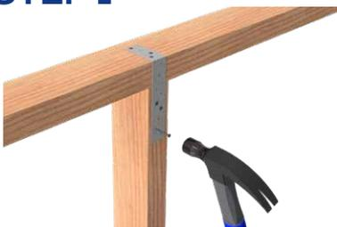
With timber frames set up, install a stud tie/flat strap (30 x 0.8mm min.) fixed to top plate and stud (This step can also be done after brace is installed)
