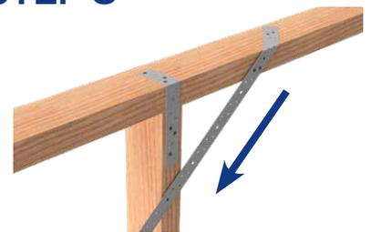
Stretch VUEBRACE at an angle of approximately 45° across the panel length of wall to be braced. Keeping in mind the acceptable panel length shall be within 1.8m to 2.7m, and the acceptable angles are between 30° to 60°.
