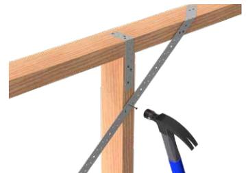
Finish by installing 1x 30mm x 2.8mm Ø VUETRADE Galvanised Timber Connector Plate Nail to every stud where brace crossed.
