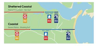
The suitability of brick ties in different environmental conditions can be determined by reading off the specification area chart based on the type of environment and the distance where the brick ties will be used.
