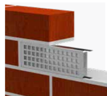
MASONRY TIES AND VENTS
